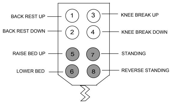
THE IONIAN STANDING BED SYSTEM IS OPERATED BY AN 8 BUTTON HANDSET.
